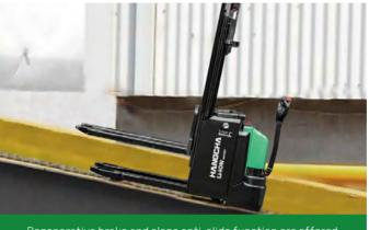
Regenerative brake and slope anti-slide function are offered by this truck
