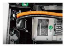
The power plug is fixed on the truck body to avoid damage from battery installment.
